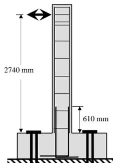
splices in square and rectangular reinforced concrete columns using combinations of CFRP jackets and CFRP anchors. Three square columns (460 mm x 460 mm x 2970 mm) and one rectangular column (460 mm x 910 mm x 2970 mm) were fabricated and rehabilitated using CFRP jackets only or by a combination of CFRP jackets and CFRP anchors. Both damaged and undamaged columns were strengthened and tested. The geometry and loading configuration for the test specimens are provided in Figure 1.
