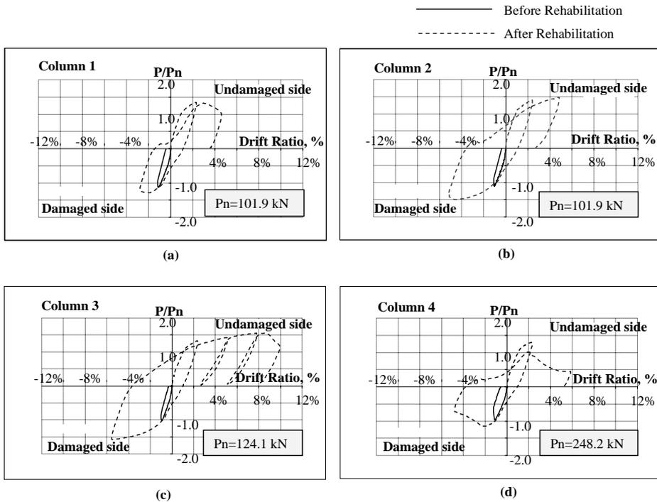
Figure 2 Drift ratio-normalized load response (a) Column 1. (b) Column 2. (c) Column 3. (d) Column 4.
