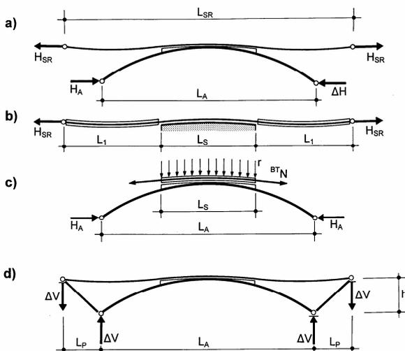
Fig. 1 Stress ribbon supported by arch
