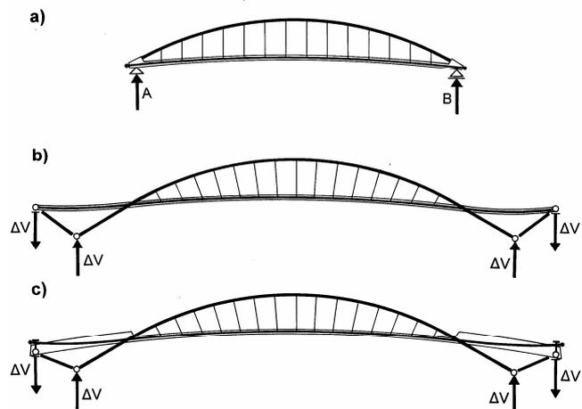
Fig. 2 Stress ribbon suspended on arch
