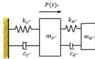
Fig. 1. TMD Schematic
