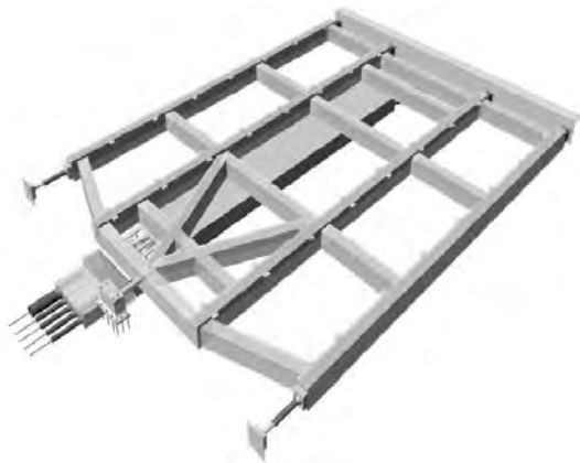
Fig. 3: Aquanect, a structural connection between floating buildings and road
