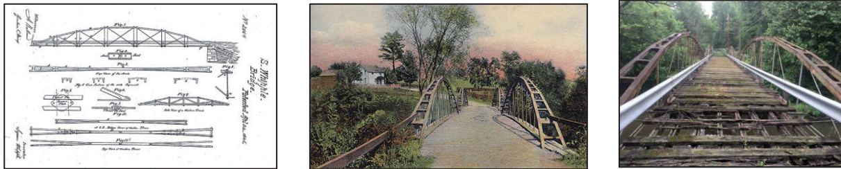
Figure 1 (a) Whipple's Bowstring Patent Drawings 1841 (b) Shaw Bridge c. 1900 (c) Shaw Bridge 2016
