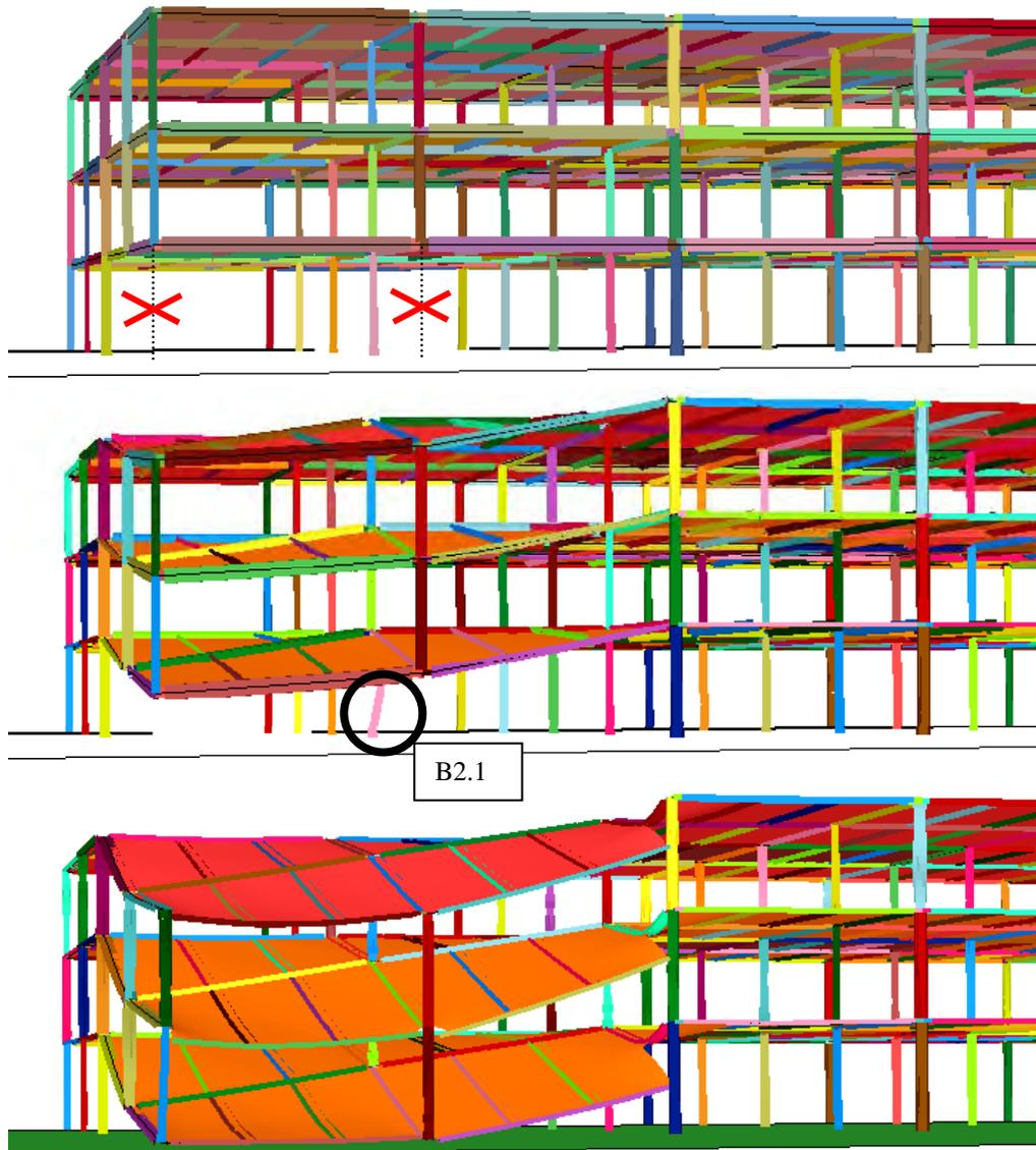
*Fig. 1: Collapse sequence of the steel building after removal of three columns*
